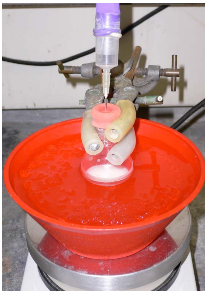
Figure 3 Boron enolate formation (end of step 15), showing precipitate of triethylamine hydrochloride.
